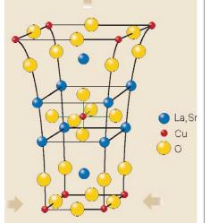
Figure 1  $La_{1,9}Sr_{0,1}CuO_{49}$  on a substrate that forces it to distort its usual crystal structure (the actual strain is exaggerated here). This distortion can increase the substance's superconducting transition temperature by a factor of two.
